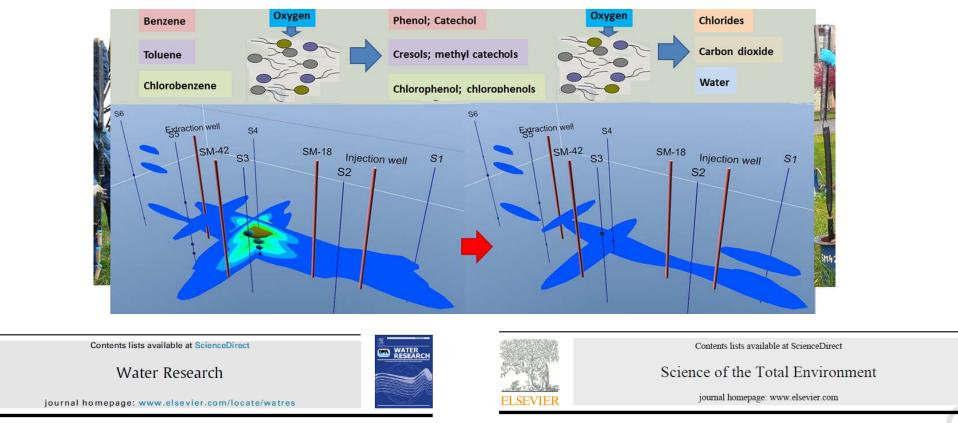
Pharmaceuticals, benzene, toluene and chlorobenzene removal from contaminated groundwater by combined UV/H<sub>2</sub>O<sub>2</sub> photo-oxidation and aeration
