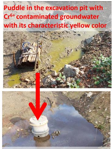
Same puddle after the injections – Cr6+ was reduced and later precipitated causing a color change
