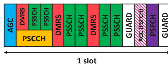
Figure 1(b) Example slot format of 3-symbol PSCCH, 3-symbol PSSCH-DMRS, and PSFCH.
